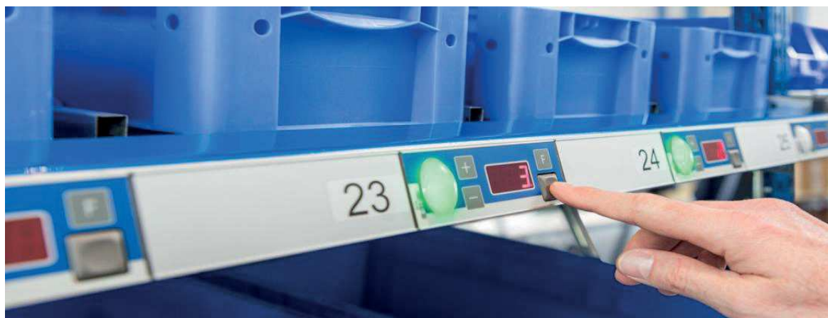
Rysunek 1. Technologia pick by light
