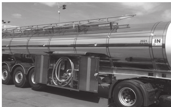
Figure 10. Open cabinet with installation for milk collection and analysis at a tanker with circular cross-section on a self-supporting semi-trailer
