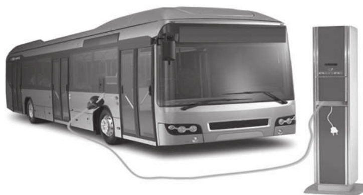
Figure 3. Electric bus charging scheme based on the plug-in connector
