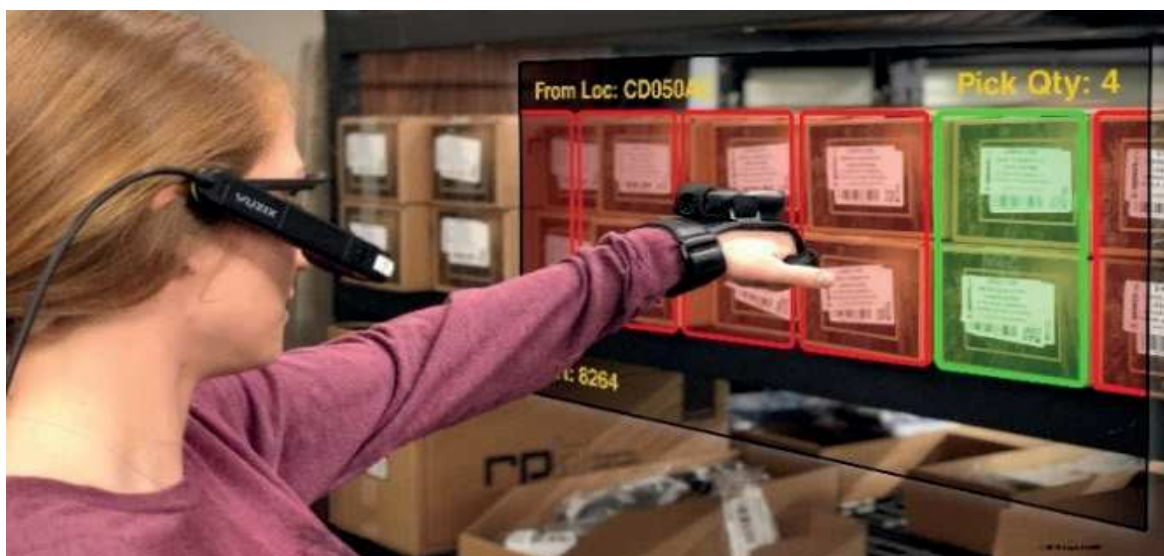
Rysunek 2. Technologia pick by vision
